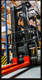
RAVAS mobile weighing allows you to transport and weigh at the same time. You immediately know the weight of every pallet lifted.
