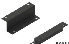
**Part #B0031** - Top Mounting Bracket set for the unheated LP2 series, Obsidian Black. One set required per air curtain. Model 84"-144" long require an additional set for center support. (Field Installed)
