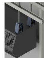
Typical overhead mounting for Spring Isolator
